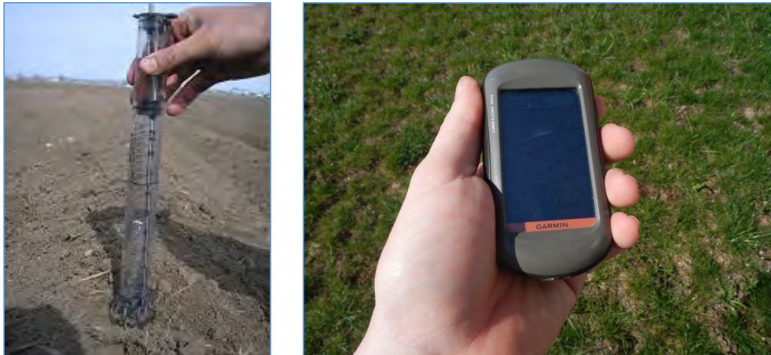
Figure 1 MiniDisc Infiltrometer (A) and GPS unit (B)
